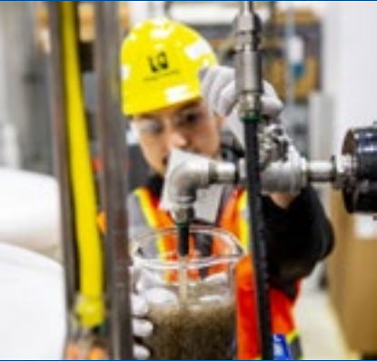
Max Armenta samples the granular sludge that will be added to the West Point Treatment Plant's existing treatment system as part of a pilot project to enable nutrient removal.
